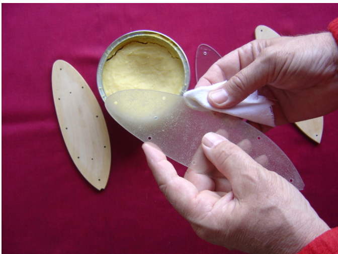
PARTS ARE TREATED WITH MOLD RELEASE WAX
