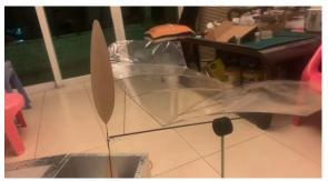
Most of the Chinese fliers use carbon fiber as the main material and use balsa sheets to build propellers. I assume this is because most of them are not familiar with balsa construction. My Black Bauhinia uses full balsa, no fiber materials; this is to encourage more fliers who do not have boron or carbon fiber materials to start building with basic materials and enter national championships.
